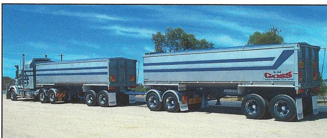
Figure 3.6: Picture of a road train with two “tipper” trailers. Source: Freightmaster Semi-trailers (Burton, South Australia)
