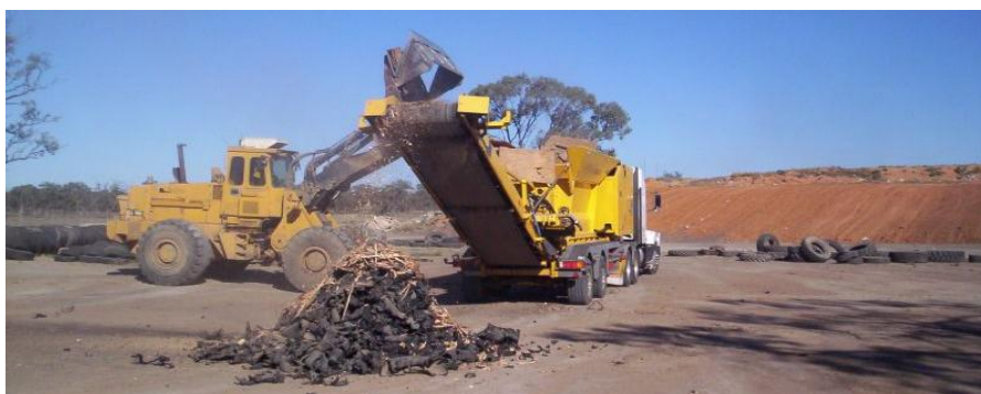
Figure 3.4: Picture of industrial-grade shredder that was employed for waste oyster basket shredding trials at Denial Bay. Source: Chris Curran, Integrated Recycling (Mildura, Victoria)
